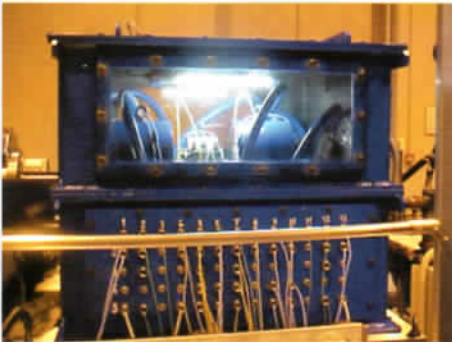
Bearing test bench at full speed and full load
